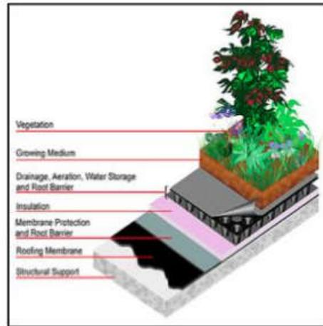
Figure 2: An overview to the conventional green roof (Dhalla and Zimmer, 2010)
